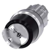
RONIS key-operated switch, 22 mm, round, metal, shiny, lock number 455, with 2 keys, 2 switch positions O-I, latching, actuating angle 90°, 10:30h/13:30h, key removal I, with laser labeling, inscription or symbol Customer-specific selection with SIRIUS ACT configurator (CIN)
