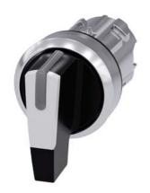
Selector switch, illuminable, 22 mm, round, metal, shiny, white, selector switch, long, 3 switch positions I>O<II, momentary contact type, actuating angle  $2x45^{\circ}$ , 10:30h/12h/13:30h, Z=50-unit packaging
