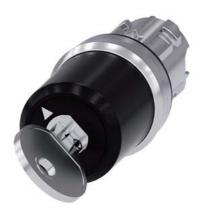
key-operated switch Siemens, 22 mm, round, metal, shiny, lock no. LSG1, with 2 keys, 2 switch positions O-I, latching, actuating angle 90°, 10:30h/13:30h, key removal O+I, with laser labeling, inscription or symbol customer-specific selection with SIRIUS ACT configurator (CIN)
