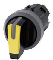
Selector switch, illuminable, 22 mm, round, plastic with metal front ring, yellow, selector switch, short, 3 switch positions I>O<II, momentary contact on the left, latching on the right, actuating angle 2x45°, 10:30h/12h/13:30h, with laser labeling, upper case and lower case, always upper case at beginning of line
