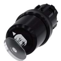
Key-operated switch BKS, 22 mm, round, plastic, lock number S1, with 2 keys, 2 switch positions O<I, momentary contact type, Actuating angle 45°, 10:30h/12h, key removal O, with laser labeling, upper case
