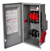
Siemens Low Voltage Circuit Protection Heavy Duty Safety Switches. Type: ENCLOSED, SAFETY SWITCH Std: UL V. Rating: 600V A. Rating: 200A No. Of Poles: 3P F. Rating: 60Hz Action: SINGLE THROW Material: 304SS Enclosure: TYPE 12. 2-3 point mounting holes. Insulation: YES O. Cycles: 8000 O. Temperature: (-20F-120F) AMBIENT TEMPERATURE Environmental Conditions: INDUSTRIAL
