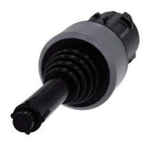
Coordinate switch, 22 mm, round, plastic with metal front ring, black, 4 switch positions, momentary contact type, with mechanical interlocking, with laser labeling, upper case and lower case, always upper case at beginning of line
