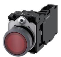
Illuminated pushbutton, 22 mm, round, plastic with metal front ring, red, pushbutton, flat, momentary contact type, with holder, 1 NO+1 NC, LED module with integrated LED 230 V AC, screw terminal, with laser labeling, upper case and lower case, always upper case at beginning of line
