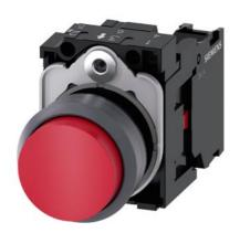
Pushbutton, 22 mm, round, plastic with metal front ring, red, pushbutton, raised, momentary contact type, with holder, 1 NC, screw terminal, with laser labeling, symbol number according to, ISO 7000 or IEC 60417
