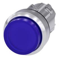
Illuminated pushbutton, 22 mm, round, metal, shiny, blue, pushbutton, raised, momentary contact type, with laser labeling, upper case and lower case, always upper case at beginning of line
