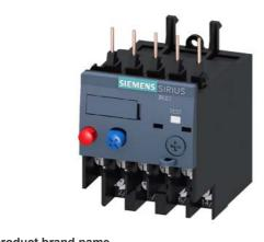
Overload relay 0.28...0.40 A Thermal For motor protection Size S00, Class 10 Contactor mounting Main circuit: Ring cable lug Auxiliary circuit: ring cable lug Manual-Automatic-Reset
