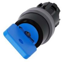
Key-operated switch O.M.R, 22 mm, round, plastic with metal front ring, lock number 73038, blue, with 2 keys, 2 switch positions O-I, latching, actuating angle 90°, 10:30h/13:30h, key removal O, Z=50-unit packaging
