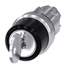
RONIS key-operated switch, 22 mm, round, metal, shiny, lock number SB30, with 2 keys, 3 switch positions I-O<II, left latching, right momentary contact type, actuating angle 2x45°, 10:30h/12h/13:30h, key removal I, possible special locks: SB31, 421, 455, Z=50-unit packaging
