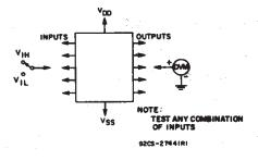
Fig. 11 - Quiescent device current test circuit.
