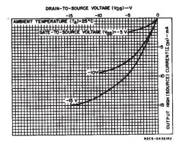
Fig. 8 - Minimum output high (source) current characteristics.
