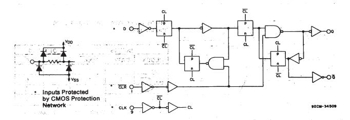
Fig. 1 - Logic diagram (1 of 4 flip-flops).
