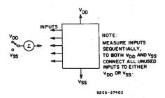
Fig. 13 - Input leakage current test circuit.
