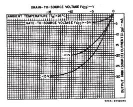
Fig. 7 – Typical output high (source) current characteristics.
