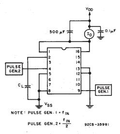
Fig. 10 - Dynamic power dissipation test circuit.
