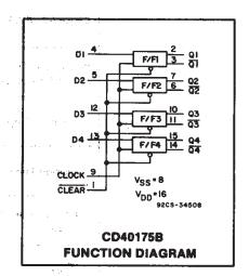
CD40175B consists of four identical D-type flipflops. Each flip-flop has an independent DATA D input and complementary Q and Q outputs. The CLOCK and CLEAR inputs are common to all flip-flops. Data are transferred to the Q outputs on the positive-going transition of the clock pulse. All four flip-flops are simultaneously reset by a low level on the CLEAR input.
