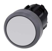
Pushbutton, 22 mm, round, plastic with metal front ring, white, pushbutton, flat momentary contact type, Z=100-unit packaging
