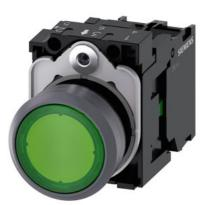
Illuminated pushbutton, 22 mm, round, plastic with metal front ring, green, pushbutton, flat, momentary contact type, with holder, 1NO, LED module with integrated LED 110 V AC, screw terminal, Z=20-unit packaging
