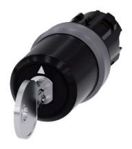
key-operated switch Siemens, 22 mm, round, plastic with metal front ring, lock number SSG10, with 2 keys, 3 switch positions I>O<II, momentary contact on the left, latching on the right, actuating angle 2x45°, 10:30h/12h/13:30h, key removal O, with laser labeling, lower case
