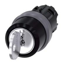
RONIS key-operated switch, 22 mm, round, plastic with metal front ring, lock number SB30, with 2 keys, 3 switch positions I-O<II, left latching, right momentary contact type, actuating angle 2x45°, 10:30h/12h/13:30h, key removal I, possible special locks: SB31, 421, 455, Z=50-unit packaging
