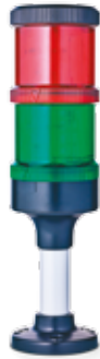
Order number: ECO70-Q02 Colours: red/green Function: LED steady beacon Nominal voltage: 24 V AC/DC Type of mounting: Tube mounting (100 mm tube length)
