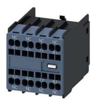
Auxiliary switch on the front, 4 NC Current path 1 NC, 1 NC, 1 NC, 1 NC for contactor relays Size S00 spring-type terminal 51/52, 61/62, 71/72, 81/82 Physically coded; only with contactor relays 3RH2140\* and 3RH2440\* can be combined (according to EN 50011)
