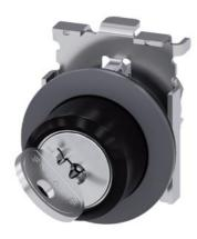
RONIS key-operated switch, 30 mm, round, Metal, matte, front ring for flush installation, lock number SB30, with 2 keys, 2 switch positions O-I, latching, actuating angle 90°, 10:30h/13:30h, key removal I, possible special locks: SB31, 421, 455, with laser labeling, upper case and lower case, always upper case at beginning of line
