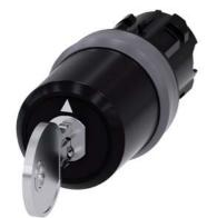
Key-operated switch BKS, 22 mm, round, plastic with metal front ring, lock number S1, with 2 keys, 3 switch positions I>O<II, momentary contact type, actuating angle 2x45°, 10:30h/12h/13:30h, key removal O, Z=50-unit packaging
