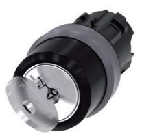
RONIS key-operated switch, 22 mm, round, plastic with metal front ring, lock number SB30, with 2 keys, 2 switch positions O-I, latching, actuating angle 90°, 10:30h/13:30h, key removal I, possible special locks: SB31, 421, 455, with laser labeling, inscription or symbol Customer-specific selection with SIRIUS ACT configurator (CIN)
