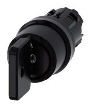
Key-operated switch O.M.R, 22 mm, round, plastic, lock number 73034, black, with 2 keys, 3 switch positions I-O-II, latching, actuating angle 2x45°, 10:30h/12h/13:30h, key removal O, with laser labeling, upper case and lower case, always upper case at the beginning of the word
