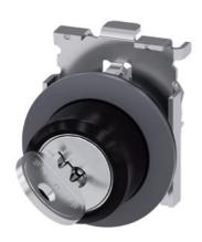
RONIS key-operated switch, 30 mm, round, Metal, matte, front ring for flush installation, lock number SB30, with 2 keys, 2 switch positions O-I, latching, actuating angle 90°, 10:30h/13:30h, key removal I, possible special locks: SB31, 421, 455, with laser labeling, upper case and lower case, always upper case at the beginning of the word
