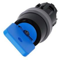
Key-operated switch O.M.R, 22 mm, round, plastic with metal front ring, lock number 73038, blue, with 2 keys, 2 switch positions O-I, latching, actuating angle 90°, 10:30h/13:30h, key removal O+I, with laser labeling, inscription or symbol Customer-specific selection with SIRIUS ACT configurator (CIN)
