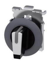
Selector switch, illuminable, 30 mm, round, Metal, matte, white, selector switch, short, front ring for flush installation, 3 switch positions I-O-II, latching, actuating angle 2x45°, 10:30h/12h/13:30h, with laser labeling, lower case
