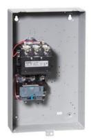
Non-reversing motor starter, Size 3 1/2, Three phase full voltage, Solidstate overload relay, OLR amp range 50-200A, Non-combination type, Enclosure type 1, Indoor general purpose use, Standard width enclosure
