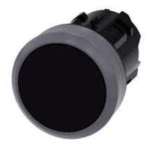
Pushbutton, 22 mm, round, plastic with metal front ring, black, pushbutton, flat, latching, Push-to-release mechanism, with laser labeling, inscription or symbol Customer-specific selection with SIRIUS ACT configurator (CIN)
