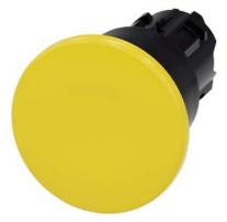
Mushroom pushbutton, 22 mm, round, plastic, yellow, 40mm, latching, pull-to-unlatch mechanism, with laser labeling, inscription or symbol Customer-specific selection with SIRIUS ACT configurator (CIN)
