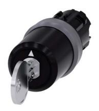
Key-operated switch BKS, 22 mm, round, plastic with metal front ring, lock number S1, with 2 keys, 3 switch positions I-O-II, latching, actuating angle  $2x45^{\circ}$ , 10:30h/12h/13:30h, Key removal I+II, with laser labeling, upper case and lower case, always upper case at beginning of line
