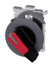
Selector switch, illuminable, 30 mm, round, Metal, matte, red, selector switch, long, front ring for flush installation, 2 switch positions O<I, momentary contact type, Actuating angle 45°, 10:30h/12h, with laser labeling, upper case
