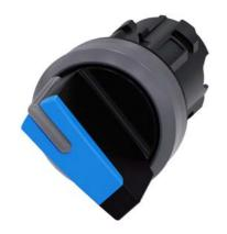
Selector switch, illuminable, 22 mm, round, plastic with metal front ring, blue, selector switch, short, 2 switch positions O<I, momentary contact type, Actuating angle 45°, 10:30h/12h, with laser labeling, upper case and lower case, always upper case at beginning of line
