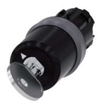
Key-operated switch BKS, 22 mm, round, plastic with metal front ring, Lock No. E7 (VW), without key, 2 switch positions O-I, latching, actuating angle 90°, 10:30h/13:30h, key removal O, with laser labeling, inscription or symbol Customer-specific selection with SIRIUS ACT configurator (CIN)
