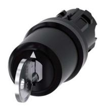
Key-operated switch IKON, 22 mm, round, plastic, lock number 360012K1, with 2 keys, 3 switch positions I-O<II, left latching, right momentary contact type, actuating angle 2x45°, 10:30h/12h/13:30h, key removal O+I, with laser labeling, upper case
