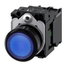
Illuminated pushbutton, 22 mm, round, plastic, blue, pushbutton, flat, momentary contact type, with holder, 1NO, LED module with integrated LED 230 V AC, screw terminal, with laser labeling, upper case and lower case, always upper case at beginning of line
