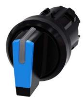
Selector switch, illuminable, 22 mm, round, plastic, blue, selector switch, short, 3 switch positions I>O<II, momentary contact type, actuating angle 2x45°, 10:30h/12h/13:30h Z=50-unit packaging
