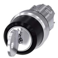
RONIS key-operated switch, 22 mm, round, metal, shiny, lock number SB30, with 2 keys, 3 switch positions I-O-II, latching, actuating angle 2x45°, 10:30h/12h/13:30h, Key removal I+O+II, possible special locks: SB31, 421, 455, with laser labeling, upper case
