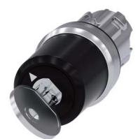
Key-operated switch BKS, 22 mm, round, metal, shiny, Lock No. E9 (VW), without key, 2 switch positions O-I, latching, actuating angle  $90^{\circ}$ , 10:30h/13:30h, key removal O+I, with laser labeling, lower case
