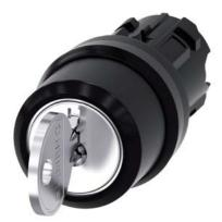
RONIS key-operated switch, 22 mm, round, plastic, lock number SB30, with 2 keys, 3 switch positions I-O<II, left latching, right momentary contact type, actuating angle 2x45°, 10:30h/12h/13:30h, key removal O+I, possible special locks: SB31, 421, 455, with laser labeling, upper case and lower case, always upper case at the beginning of the word
