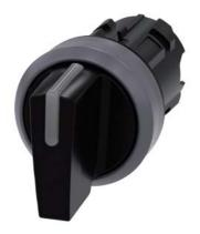
Illuminable selector switch, 22 mm, round, plastic with metal front ring, black, Selector switch short, 3 switch positions I>O<II, momentary contact on the left, latching on the right, actuating angle  $2x45^{\circ}$ , 10:30 /12 /13:30, Z=50-unit packaging
