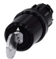
key-operated switch Siemens, 22 mm, round, plastic, lock number SSG10, with 2 keys, 3 switch positions I-O<II, left latching, momentary contact type on the right, actuating angle  $2x45^{\circ}$ , 10:30h/12h/13:30h, key removal I, with laser labeling, upper case
