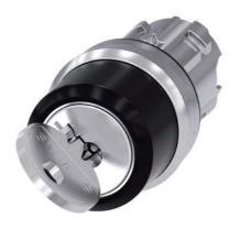
RONIS key-operated switch, 22 mm, round, metal, shiny, Lock No. 421, with 2 keys, 2 switch positions O-I, latching, actuating angle  $90^{\circ}$ , 10:30h/13:30h, key removal O+I, with laser labeling, upper case and lower case, always upper case at the beginning of the word
