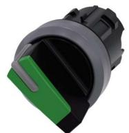
Selector switch, illuminable, 22 mm, round, plastic with metal front ring, green, selector switch, short, 2 switch positions O-I, latching, actuating angle 90°, 10:30h/13:30h, with laser labeling, upper case and lower case, always upper case at the beginning of the word
