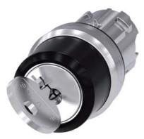
RONIS key-operated switch, 22 mm, round, metal, shiny, Lock No. 421, with 2 keys, 2 switch positions O-I, latching, actuating angle  $90^\circ$ , 10:30h/13:30h, key removal O+I, with laser labeling, upper case
