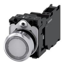
Illuminated pushbutton, 22 mm, round, Metal, shiny, transparent, pushbutton, flat, momentary contact type, with holder, 1 NO+1 NC, LED module with integrated LED 230 V AC, spring-type terminal, with laser labeling, symbol number according to, ISO 7000 or IEC 60417
