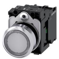
Illuminated pushbutton, 22 mm, round, metal, shiny, clear, pushbutton, flat, momentary contact type, with holder, 1NO, LED module with integrated LED 24 V AC/DC, screw terminal, Z=20-unit packaging
