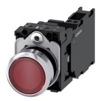
Illuminated pushbutton, 22 mm, round, Metal, shiny, red, pushbutton, flat, momentary contact type, with holder, 1 NO+1 NC, LED module with integrated LED 230 V AC, spring-type terminal, with laser labeling, lower case
