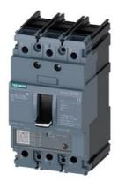
circuit breaker 3VA5 UL frame 125 3-pole, starter protection TM120M, AM, In=7A without overload protection short-circuit protection Ii=3...7 x In nut keeper kit on both sides
