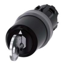
Key-operated switch IKON, 22 mm, round, plastic with metal front ring, lock number 360012K1, with 2 keys, 3 switch positions I-O<II, left latching, right momentary contact type, actuating angle 2x45°, 10:30h/12h/13:30h, key removal O+I, with laser labeling, upper case and lower case, always upper case at beginning of line
